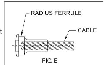
**B. Place Ferrule, Radius Ferrule, or stud into open swager dies.**
