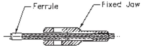
2. Grasp top of Clip with pliers, and force clip over cable immediately behind Ferrule.
