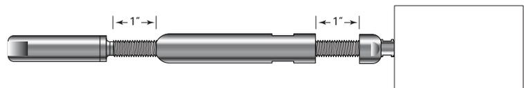
2. Mark the Push-Lock stud body at 1-3/16" from the cable entrance of the stud. Holding the fitting, pull the cable taut over the mark on the stud and transfer the mark to the cable. Cut cable at mark.
