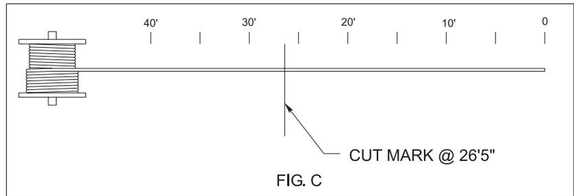
**NOTE:** Make sure you have a positive holding device at the zero end. Cutting the cables takes very little time. It is best to have one person stand at the zero mark while the other operates the cable cutter at the cut mark.
