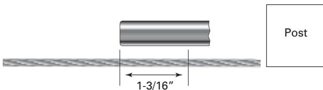
4. Detach the tensioning device from the cable at the other end of the run to allow cable slack so you can perform the next step.
