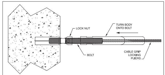
**\*NOTE:** This will allow for maximum take-up. The fewer turns you make at this step, the more thread that will be exposed when the installation is complete. Each job is different, so we suggest that you string and lightly tension one cable between end posts, to determine how many turns you will make in turning the body onto the male threaded end in order to minimize the amount of exposed thread at both ends.
