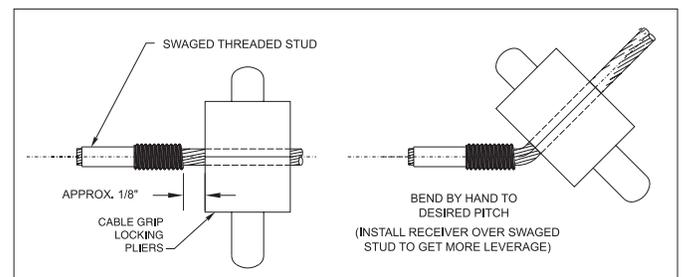
**5. Install the Receiver** in the post, following the instructions for installing Invisiware® Receivers at Post B in the "Installing Cable" on pages 4-9. When tensioned, the cables will self-align with the fitting at the other end of the cable run.
