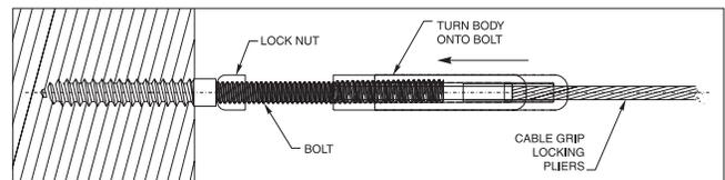
If you are installing into a threaded hole in a metal post, screw the bolt into the threaded hole in the post. Screw the lock nut onto the threads of the bolt, then hold the cable closely behind the body and turn the body by hand onto the threaded end of the bolt at least 6 full turns.
