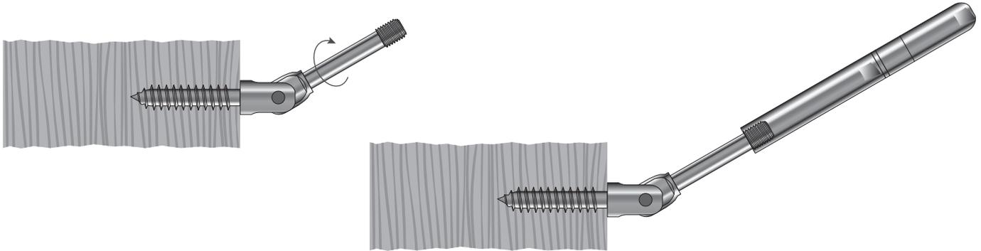
**2C.** If you are using the Push-Lock Tensioner with Threaded Bolt, hand turn the threaded bolt component of the assembly clockwise into the post, tightening with a 3/16" hex wrench. Assemble female threaded rotating portion of fitting onto male thread only so far as to cover the male thread and no more.
