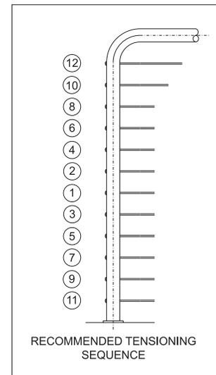
6. Return to Post B and finish tensioning using the Turnbuckle. While preventing the Push-Lock stud from turning by holding it in place with a 3/8" open-end wrench (using wrench flat), turn the body of the Turnbuckle with a 7/16" wrench until the cable is suitably tensioned. Once tensioned, there may be 1/2"-3/4" of thread left showing on either side of the Turnbuckle body. Any remaining visible thread may be needed for future tightening.
