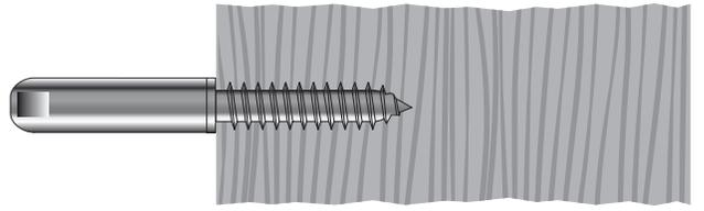
**2D.** If you are using the Push-Lock Threaded Bolt, place a black Delrin® washer over the threaded bolt. Turn the fitting into the pre-drilled and tapped 5/16-24 hole in the post using 3/8" open-end wrench on wrench flats milled into body of fitting. Stop turning when shoulder on fitting between threaded bolt and body makes contact with metal post.
