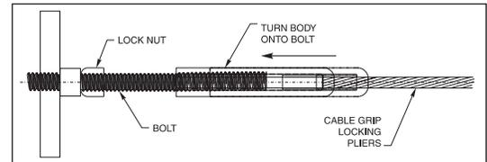
If you are installing an Adjust-A-Body concrete anchor bolt end into a concrete anchor bolt, screw the bolt into the threaded hole in the anchor bolt. Screw the lock nut onto the threads of the bolt, then hold the cable closely behind the body and turn the body by hand onto the threaded end of the bolt at least 6 full turns. (See note below)\*
