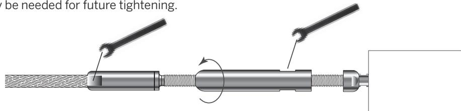
7. Remove 3/8" wrench from the Push-Lock body. Using another 7/16" wrench to prevent the Turnbuckle body from rotating, tighten the nut against the body to lock adjustment.
