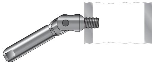
**2G.** If you are using a Push-Lock Anchor Bolt, make sure the Red Head® anchor is properly installed into the concrete per the manufacturer's specifications. Once your Red Head is in place, simply thread the fitting into the Red Head anchor until tight.
