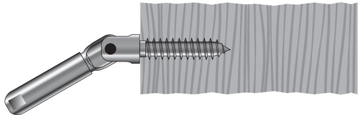
**2F.** If you are using a Push-Lock Threaded Clevis, hand turn the fitting into the pre-drilled and tapped 5/16-24 hole in the post using the articulating portion of the fitting as a lever to rotate the threaded end of fitting. Stop turning when shoulder on fitting between the thread and clevis makes contact with the metal post face. You may continue to rotate fitting up to 1/4 turn to properly orient the fitting.
