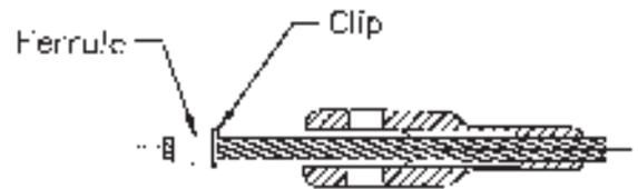
3. Pull cable back through throat of Fixed Jaw until it stops. Ferrule is captured inside Fixed Jaw.
