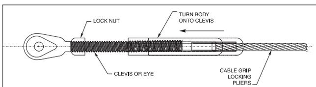
If you are installing into wood with a hanger bolt, screw the hanger bolt into a pre-drilled pilot hole in the post. Screw the lock nut onto the threads of the bolt, then hold the cable closely behind the body and turn the body by hand at least 6 full turns onto the threaded end of the bolt. (See note below)\*
