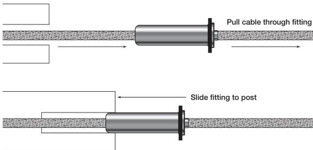
**Note:** If you have trouble inserting the cable into the fitting, it may be because the locking wedges have become stuck. This is not a defect! Here's what you can do to "free the wedges" —
