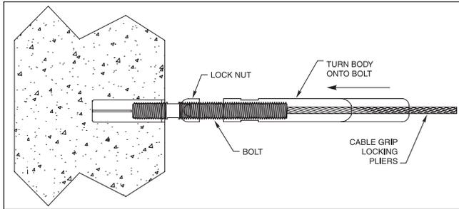
4. Repeat the above steps for each cable to be installed. Do not tension the cables, until all cables have been installed between end posts A and B.
