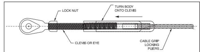
If you are installing into wood with a hanger bolt, screw the hanger bolt into a pre-drilled pilot hole in the post. Screw the lock nut onto the threads of the bolt, then hold the cable closely behind the body and turn the body by hand onto the threaded end of the bolt at least 6 full turns.
