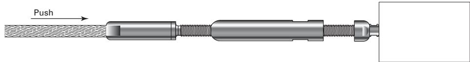
5. Reattach the tensioning device at the other end. Tension all cables in sequence, beginning with the center cables, moving up and down toward top and bottom. As you tension each cable, give it a sharp pull downward mid-span to help set the wedges, then re-tension as necessary in the same sequence. Be aware that the cable may move as much as 3/16" toward the tensioning terminal as the wedges seat.
