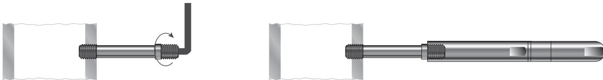
**2D.** If you are using the Push-Lock Tensioner with Threaded Clevis, hand turn the threaded clevis into the post using the articulating portion of the fitting as a lever to rotate the part. Tighten such that the unattached arm hangs vertically. Assemble female threaded rotating portion of fitting onto male thread only so far as to cover the male thread and no more.
