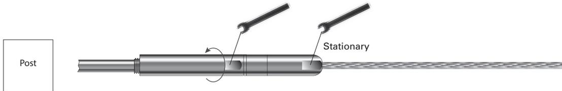
5. Tension all cables in sequence, beginning with the center cables, moving up and down toward the top and bottom. As you tension each cable, give it a sharp pull downward mid-span to help set the wedges, then re-tension as necessary in the same sequence. Be aware that the cable may move as much as 3/16" toward the tensioning terminal as the wedges seat.
