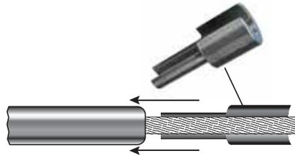
2. Push down until the key bottoms out. You will feel resistance from the spring-loaded jaws as you do so.
