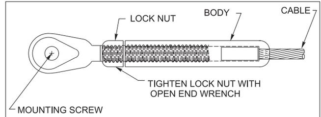
7. **On all installations, tighten the lock nut against the body of the fitting with an open-end wrench.**
