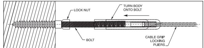
If you are installing into a threaded hole in a metal post, screw the bolt into the threaded hole in the post. Screw the lock nut onto the threads of the bolt, then hold the cable closely behind the body and turn the body by hand at least 6 full turns onto the threaded end of the bolt. (See note below)\*
