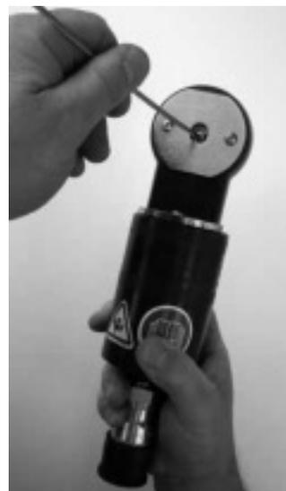
**610 Portable Swager for use with 1/8" and 3/16" diameter cable.**
