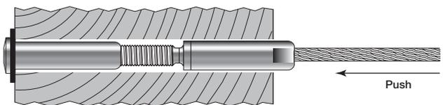
**Step B. Install the Pull-Lock® fitting on Post B.**
