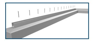
5. Open a pack of 10 mechanisms and locate the nonclamping rocker mechanism. The rocker mechanism has a single large isolator pad attached to it. 6. Snap a rocker mechanism into the far side of the shoe channel at least every 12". Each panel of glass should be supported by at least 2 mechanisms.
