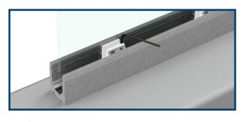
12. Install end caps on any exposed ends of the base shoe.
