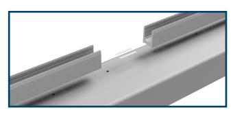
4. Base shoe isolator pads are required to protect the glass from contacting the shoe and anchor heads. Install the base shoe isolator pads (found in the pack of mechanisms) at least every 12".
