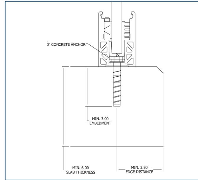
**Hollow Steel Tube without Weld Blocks**
