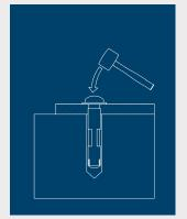
Drive the anchor through the mounting flange into the hole until the head is firmly seated. Use a rubber mallet.
