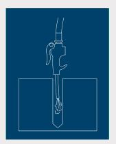
Blow the hole clean of dust and other material. Do not expand the anchor prior to installation.
