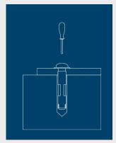
Tighten the anchor by turning the head 3 to 5 turns past finger tight or by applying the guide installation torque from the finger tight position.
