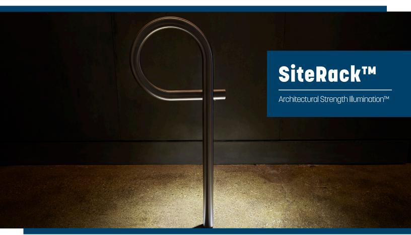
This SiteRack bicycle parking rack features a point source luminaire integrated into its sculptural, 316 stainless steel form. The 1.90" schedule 40 material and full weld mounting plate or embed, provide a robust structure to secure any type of cycle. With illumination for safety and site way-finding, the LED fixture has reliable performance with a 70° optic at nadir. The symmetric output provides a pool of illumination next to the rack and reflects across its main post surface.
