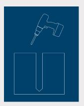
Using a 9/16th diameter bit, drill a hole into the base material to a depth at least 1/2" deeper than the required 4".
