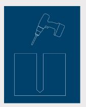
Using a 9/16th diameter bit, drill a hole into the base material to a depth at least 1/2" deeper than the required 4".
