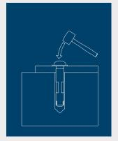
Drive the anchor through the mounting flange into the hole until the head is firmly seated. Use a rubber mallet.
